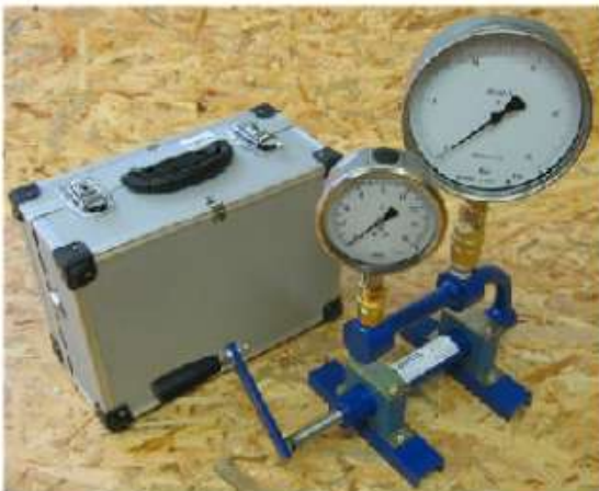
Fig. 3: Pressure balance with screw pump and calibrated pressure gauge
