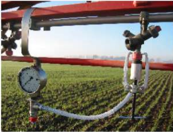
Fig. 5: Optionally available adapter with test pressure gauge for testing the pressure drop on the nozzle bar.
