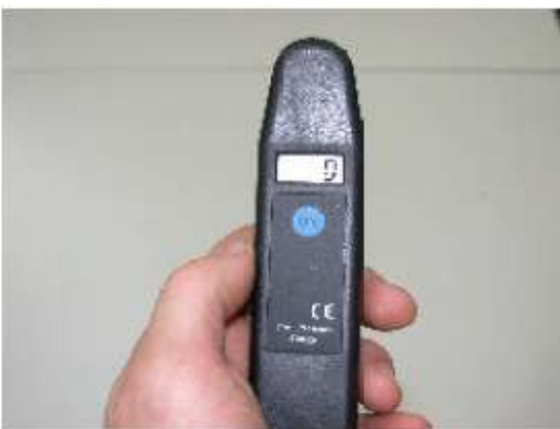
Fig. 8: Air pressure measuring device for checking the air chamber pressure on pumps.
