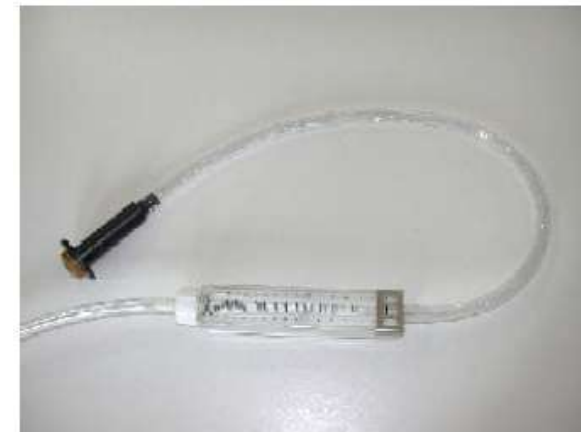
Fig. 6 and 7: Floating body flow meter for the rough estimation of individual nozzle flow volumes.
