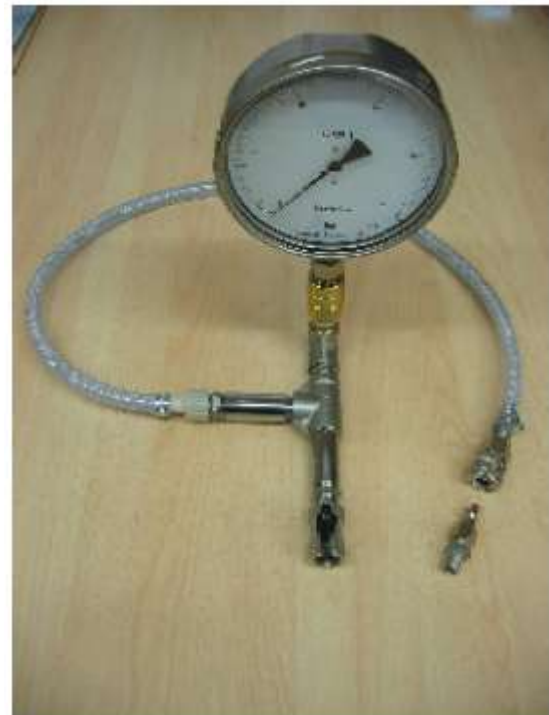
Fig. 4: The test pressure gauge can be connected to the test samples via a hose.
