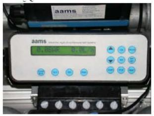
Fig. 3: Terminal with measured value indicator and function keys (touch-sensitive keyboard).
