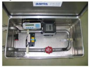
Fig. 2: Opened case with pipe, connections, flow meter and measured value indicator.
