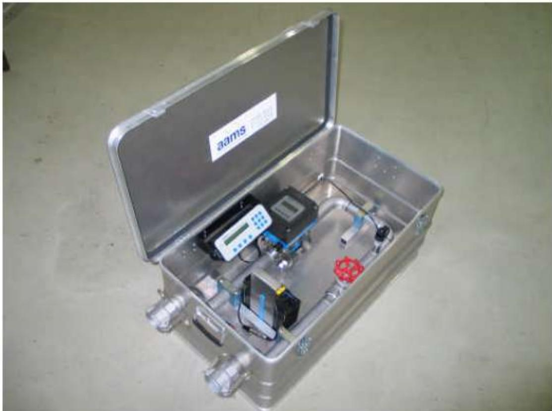
**Inspection equipment, AAMS PTP 400-16 pump testing equipment**
