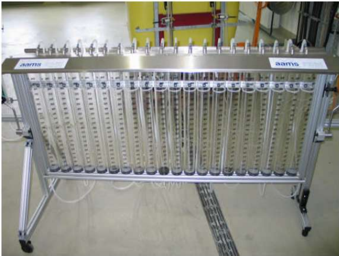
Inspection equipment Test stand for individual nozzles AAMS FRMC 16
