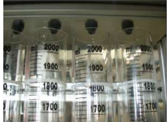
Fig. 6: Measuring cylinders with stuck-on scales
