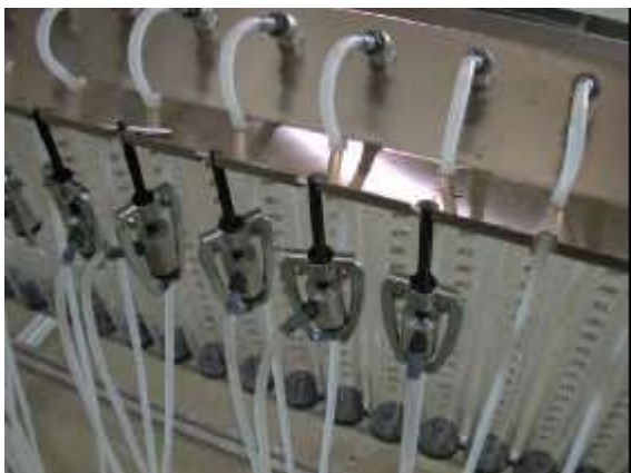
Fig. 3: Mountings for the nozzle adapters
