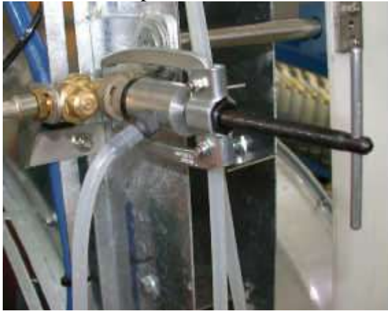
Fig. 2: Universal individual nozzle adapter
