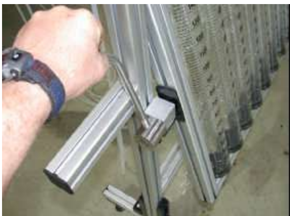
Fig. 4: Swivelling lever for filling, reading and emptying the cylinder. This is the filling position.
